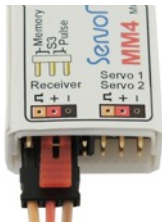
Position Pulse (right) S3 as pushbutton
